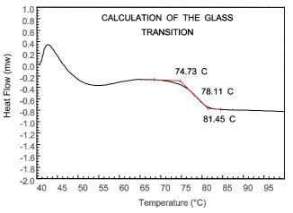
The glass transition temperature (Tg) of a polymer is the temperature range at which the polymer transitions from a rigid "glass" state to a flexible "rubber" state, affecting its usability, especially in elastomers. Understanding Tg is crucial for quality control, optimizing processes, ensuring product performance, and maintaining material consistency.
