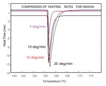
Endothermic Peak (Melting) refers to the phenomenon where a material absorbs heat and undergoes a phase transition during heating in thermal analysis. It typically appears as a distinct temperature peak, reflecting the material's melting temperature and thermal properties. The shape and width of the peak indicate the sample's purity, with pure crystalline materials displaying sharp peaks. Slower heating rates can further enhance the clarity of the peak.
