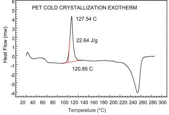
The growth and degree of crystallization of the crystals depend on the type of polymer, cooling rate, and isothermal aging time. The calculation method for crystallization enthalpy is the same as for melting enthalpy. Cold crystallization is the process in which crystals grow upon heating. This exothermic process occurs prior to crystallization melting.
